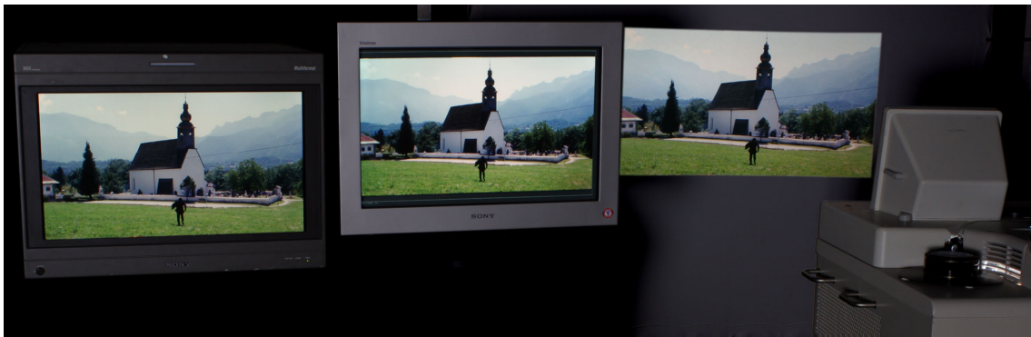
A good way to check the result of the color management: side by side projection of Sony BVM-D24E1WE (grade one monitor), Sony GDM-VW 900 (computer monitor) and film projection with ARRI Locpro Xenon.
